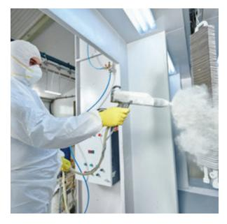
Teflon<sup>™</sup> products are generally applied by commercial spray techniques. This must be done in a hood or well-ventilated area to prevent fluoropolymers or solvent fumes from affecting breathing air of employees. See Safe Handling Fact Sheet for respirator recommendations. Separate spray guns should be used for water based and solvent-based products.
