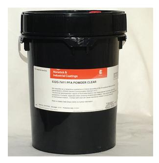
Teflon<sup>™</sup> powder coatings are free-flowing powders which are applied with conventional electrostatic powder equipment, with either spray guns or fluidised bed. The application voltage and technique depends on the particular equipment, although the highly attractive nature of the powder permits a wide range of application voltages.
