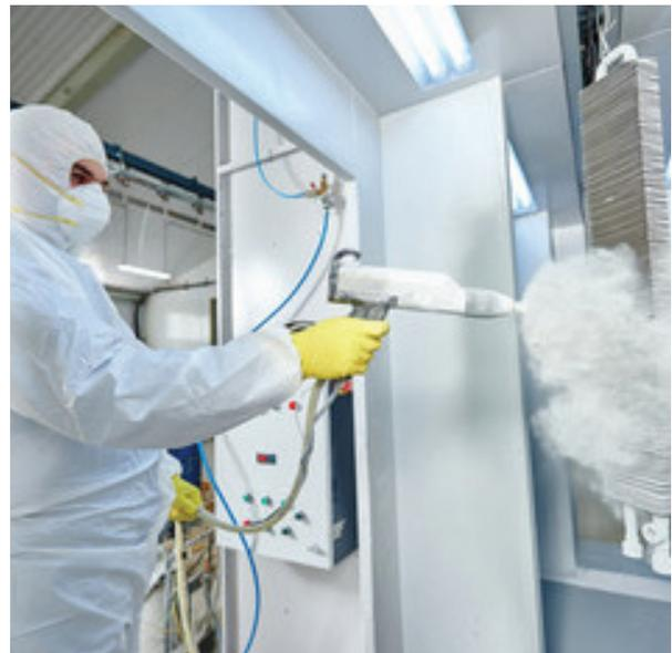
Teflon™ products are generally applied by commercial spray techniques. This must be done in a hood or well-ventilated area to prevent fluoropolymers or solvent fumes from affecting breathing air of employees. See Safe Handling Fact Sheet for respirator recommendations. Separate spray guns should be used for water based and solvent-based products.
